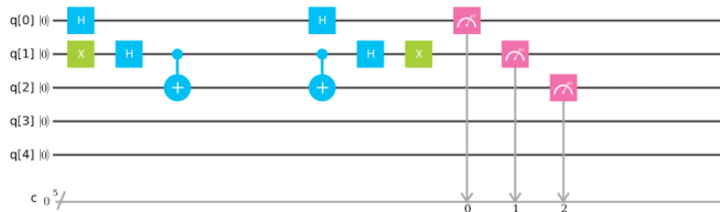
Figure 5: A quantum circuit: quantum gate operations on q-bits. Source: ibm.com
