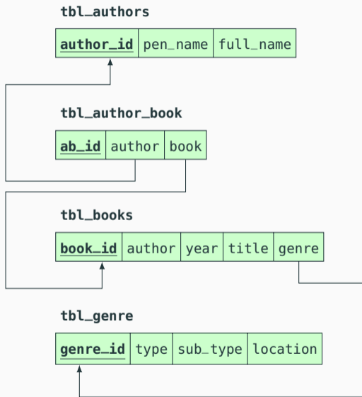
Figure 3: The improved database scheme that allows multiple authors to co-author one book by adding a table tbl_author_book
